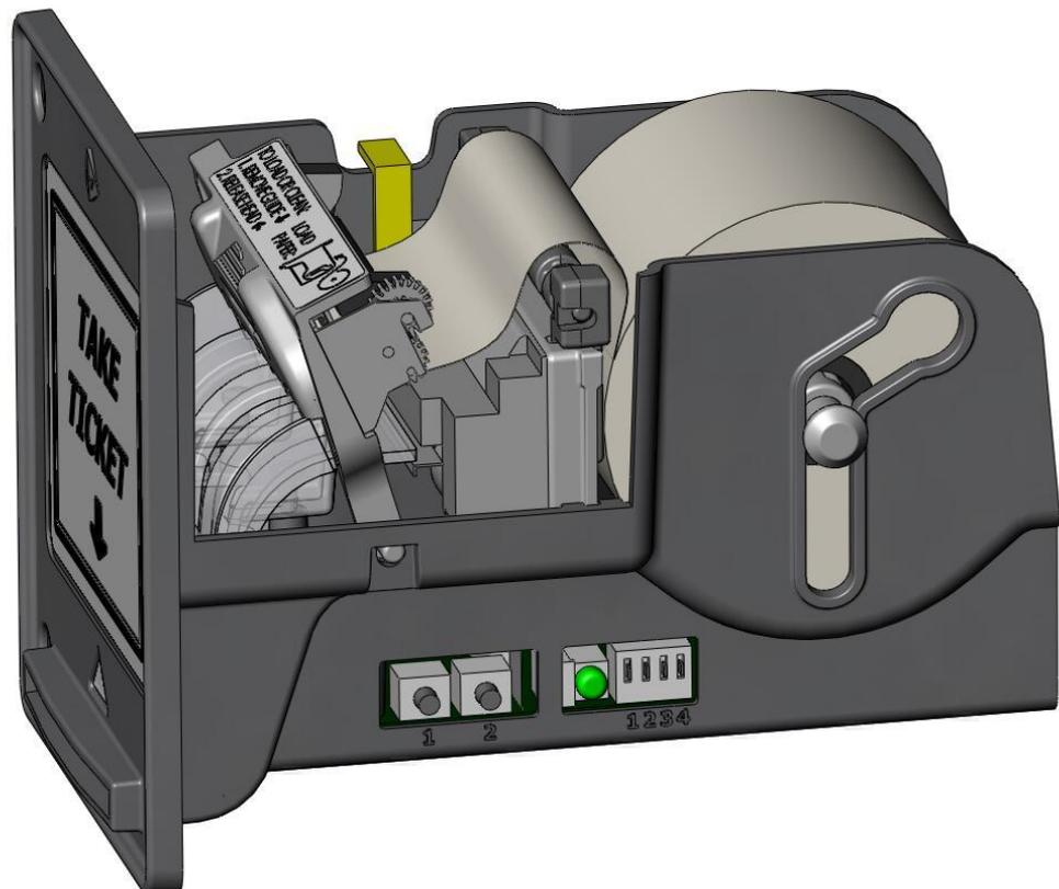
**Second Method:** (See Figure 2) cut or rip the end of the paper roll so that a nice flat edge is present. Hold this edge into the head mechanism. In a few seconds, the head will slowly pull in the paper. It will then speed up and then feed out about 12 inches of paper.
